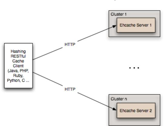
Non-redundant Scalable Cache Server Topology with client hash-based URI routing
