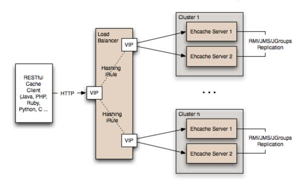
Redundant Scalable Cache Server Topology with Load Balancer hash-based URI routing
