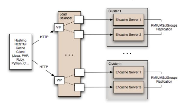
Redundant Scalable Cache Server Topology with client hash-based URI routing
