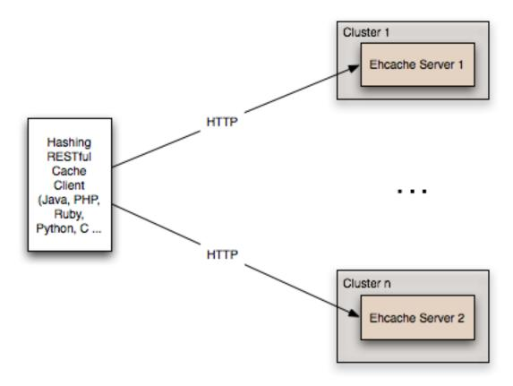
This topology is the simplest. It does not use a load balancer. Each node is accessed directly by the cache client using REST. No redundancy is provided. The client can be implemented in any language because it is simply a HTTP client. It must work out a partitioning scheme. Simple key hashing, as used by memcached, is sufficient. Here is a Java code sample:
