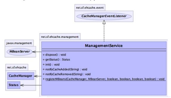
There is only one method, ManagementService.registerMBeans, which is used to initiate JMX registration of a CacheManager's instrumented MBeans. The ManagementService is a CacheManagerEventListener and is therefore notified of any new Caches added or disposed and updates the MBeanServer appropriately.
