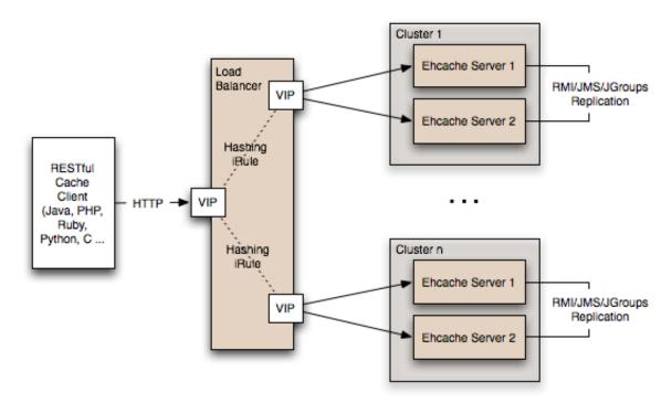
Many content-switching load balancers support URI routing using some form of regular expressions. So, you could optionally skip the client-side hashing to achieve partitioning in the load balancer itself. For example:
