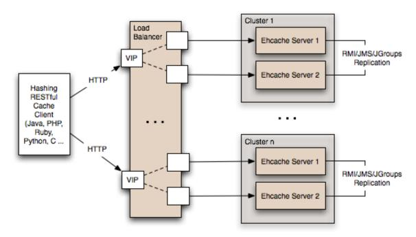
Redundancy is added as shown in the above diagram by: Replacing each node with a cluster of two nodes. One of the existing distributed caching options in Ehcache is used to form the cluster. Options in Ehcache 1.5 are RMI and JGroups-based clusters. Ehcache-1.6 will add JMS as a further option. Put each Ehcache cluster behind VIPs on a load balancer.
