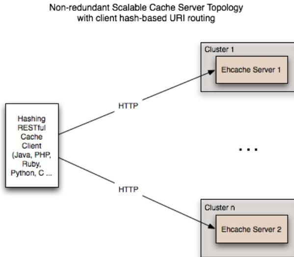
This topology is the simplest. It does not use a load balancer. Each node is accessed directly by the cache client using REST. No redundancy is provided. The client can be implemented in any language because it is simply a HTTP client. It must work out a partitioning scheme. Simple key hashing, as used by memcached, is sufficient. Here is a Java code sample:
