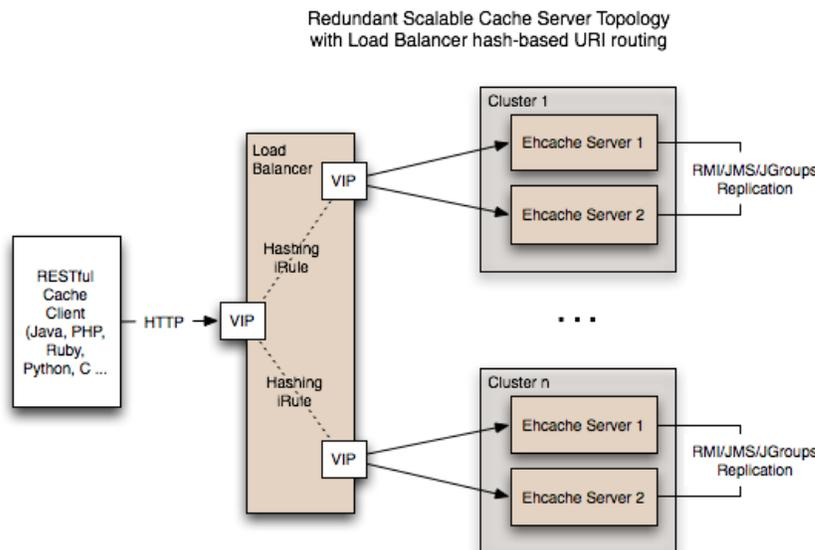
Many content-switching load balancers support URI routing using some form of regular expressions. So, you could optionally skip the client-side hashing to achieve partitioning in the load balancer itself. For example:
