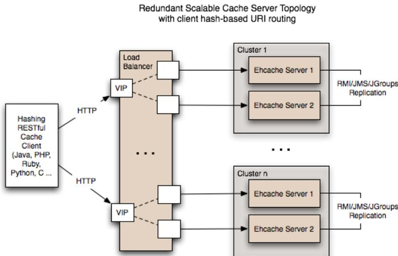
Redundancy is added as shown in the above diagram by: Replacing each node with a cluster of two nodes. One of the existing distributed caching options in Ehcache is used to form the cluster. Options in Ehcache 1.5 are RMI and JGroups-based clusters. Ehcache-1.6 will add JMS as a further option. Put each Ehcache cluster behind VIPs on a load balancer.
